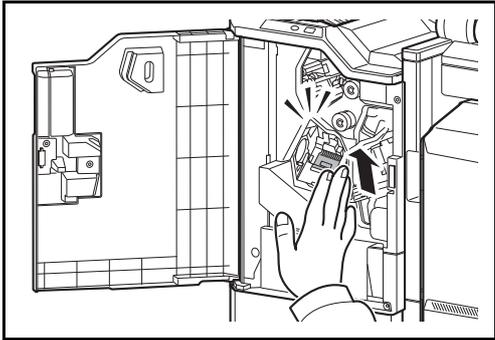
5 Re-install the staple cartridge holder. The staple cartridge holder will click into place when it has been inserted correctly.
