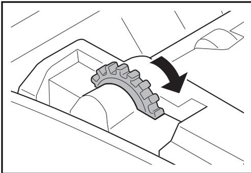
If the original is difficult to remove, turn the dial. The original will scroll out to a position where it can be removed easily.
