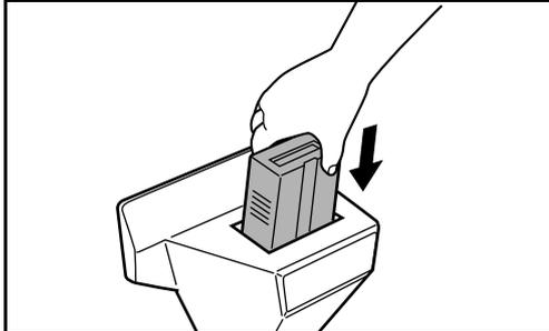
Insert the key counter securely into the key counter slot.
