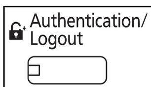
To log out the machine, press the **Authentication/Logout** key to return to the login user name/login password entry screen.
