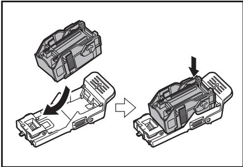
4 Insert the new staple cartridge into the staple cartridge holder.
