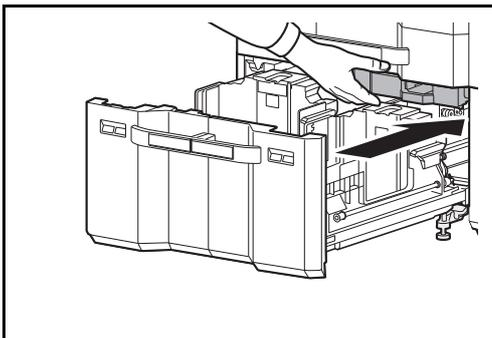
**9** Close the paper feed unit cover (B2) and push the paper feed unit all the way back in.
