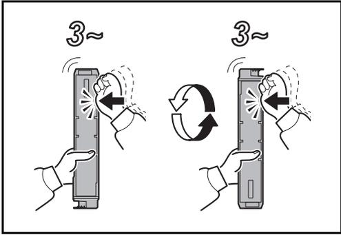
5 Hold the toner container vertically and hit the upper part about 3 times. Invert the toner container so that the other end is up, and hit in the same way.
