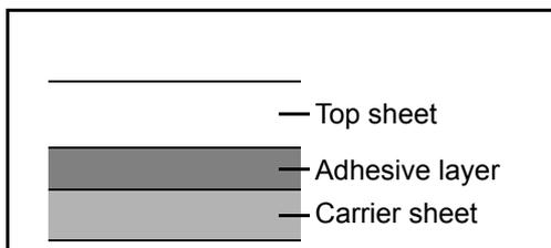
Labels consist of three layers as shown in the illustration. The adhesive layer contains materials that are easily affected by the force applied in the machine. The carrier sheet bears the top sheet until the label is used. This composition of labels may cause more problems.
