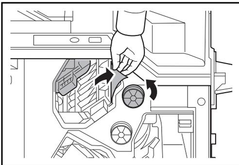
**3** Turn the conveyor knob (D3) to the left to feed the paper along to enable easy removal.
