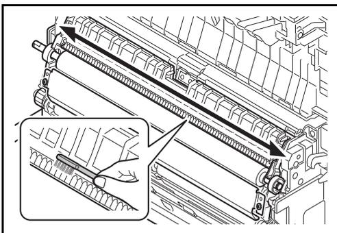
**4** As shown in the figure, clean dirt from the separator by moving the brush from side to side along the separator.
