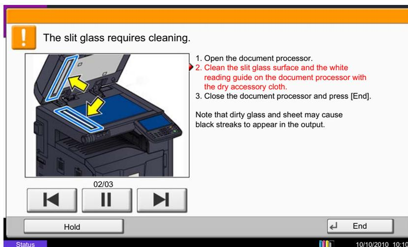
**NOTE:** Wipe the slit glasses with the dry accessory cloth. Do not use water, soap or solvents for cleaning.
