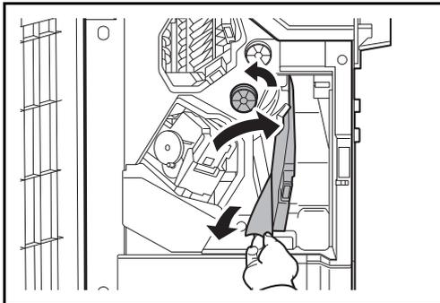
**2** Open the conveyor guide (D7) and remove the jammed paper.
