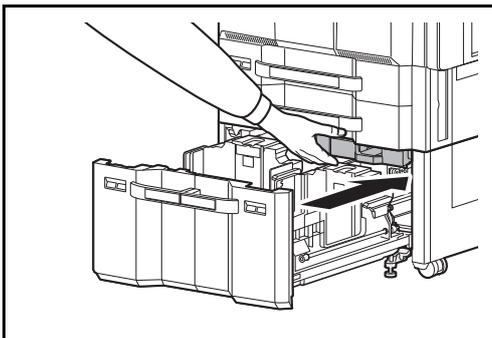
**8** Close the paper feed unit cover (B2) and push the paper feed unit all the way back in.
