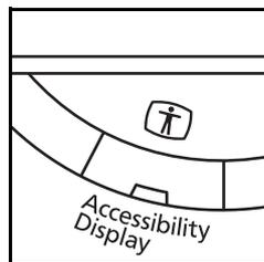
Press the **Accessibility Display** key when in the Copy or Send (i.e. the **Copy** or **Send** key indicator is On).
