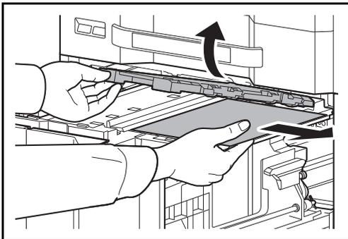
**7** Open the paper feed unit cover (B2) and remove the jammed paper.
