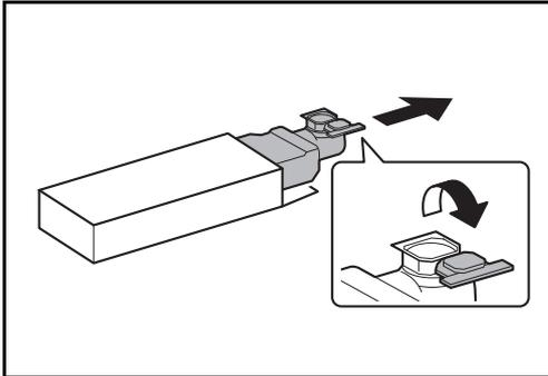
**5** Gently remove the new waste toner box from its packaging and open the cap.
