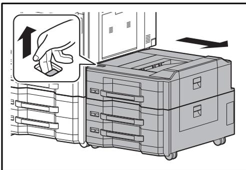
**1** Pull up the release lever and separate the side feeder from the multifunction machine.
