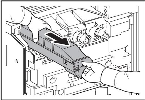
3 Remove the toner container and insert it into the provided plastic disposal bag.
