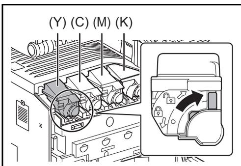
**2** Turn the toner container release lever to the vertical position.
