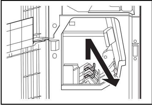
2 Remove the staple cartridge holder B or C.
