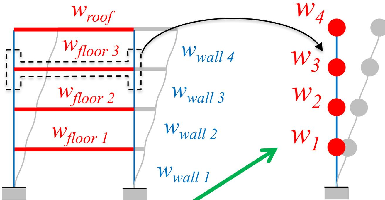
Weight of building is lumped at floor levels
