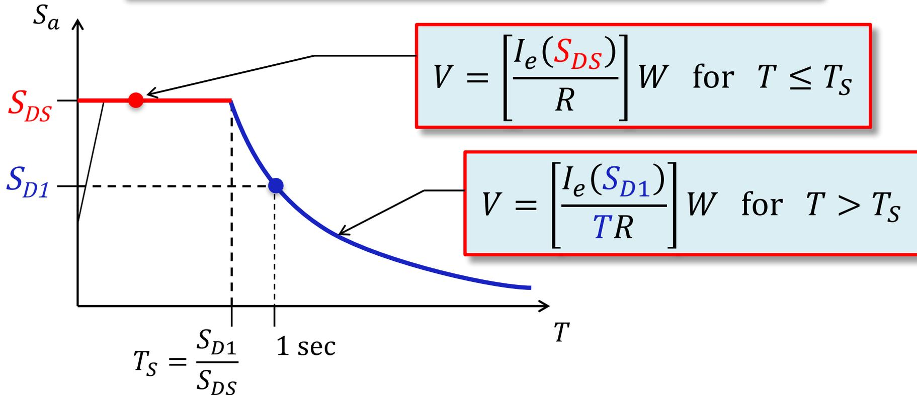
Seismic Base Shear ( $V$ ) depends on:
