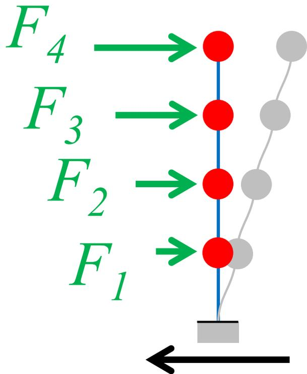
Seismic Base Shear
