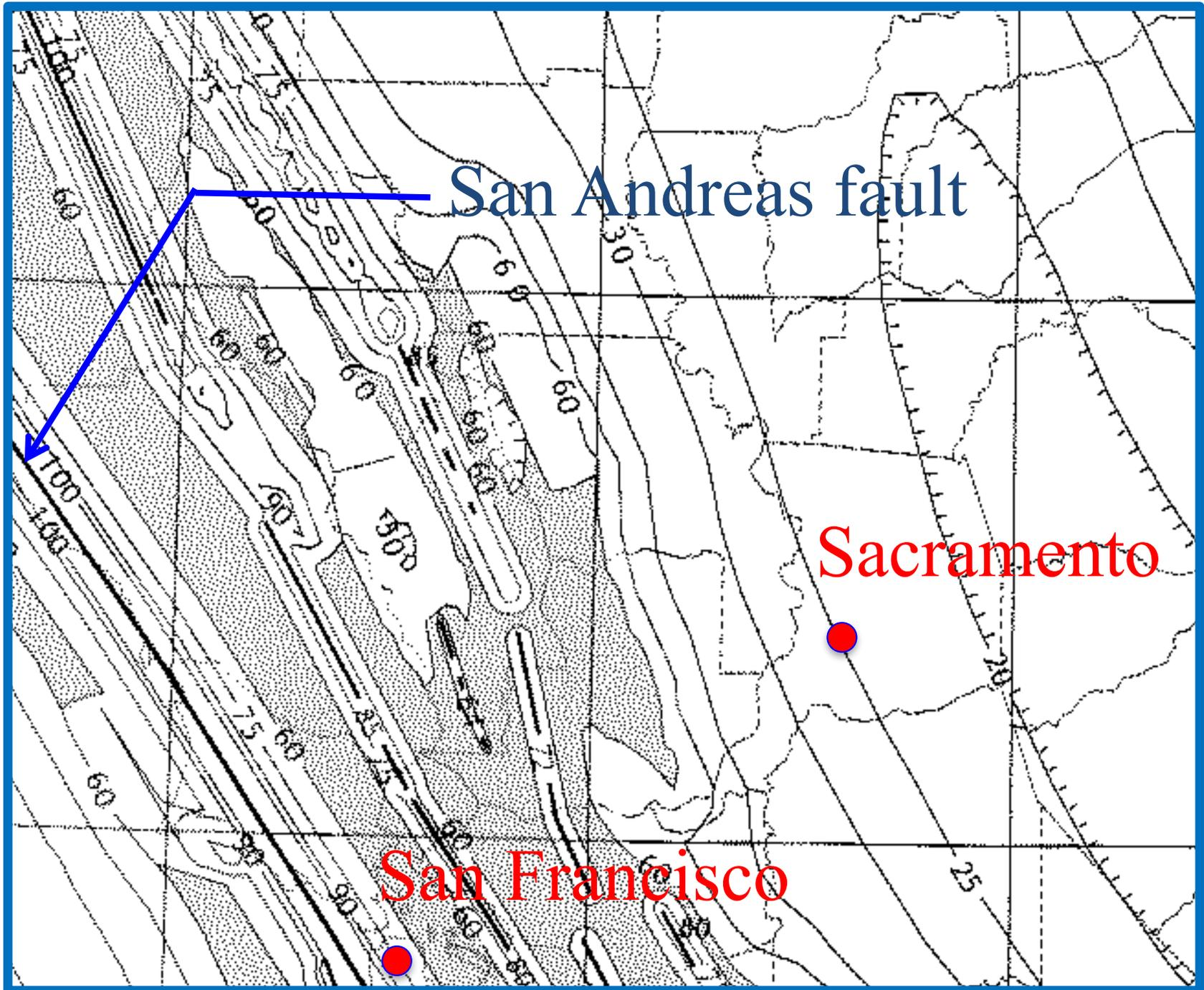
Maximum credible acceleration at the foundation of the building depends on the seismicity and the soil at the site
