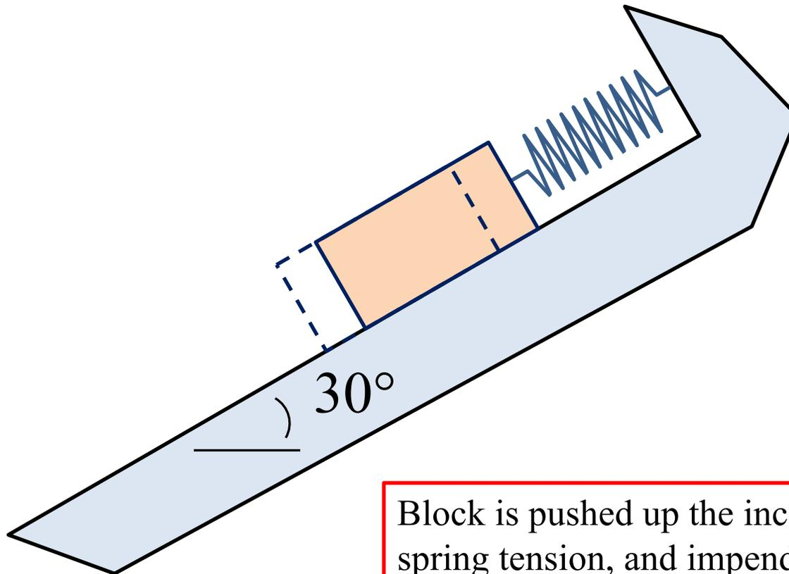
Block is pushed up the incline, decreasing spring tension, and impending motion would be for the weight of the crate to move the crate down the incline.
