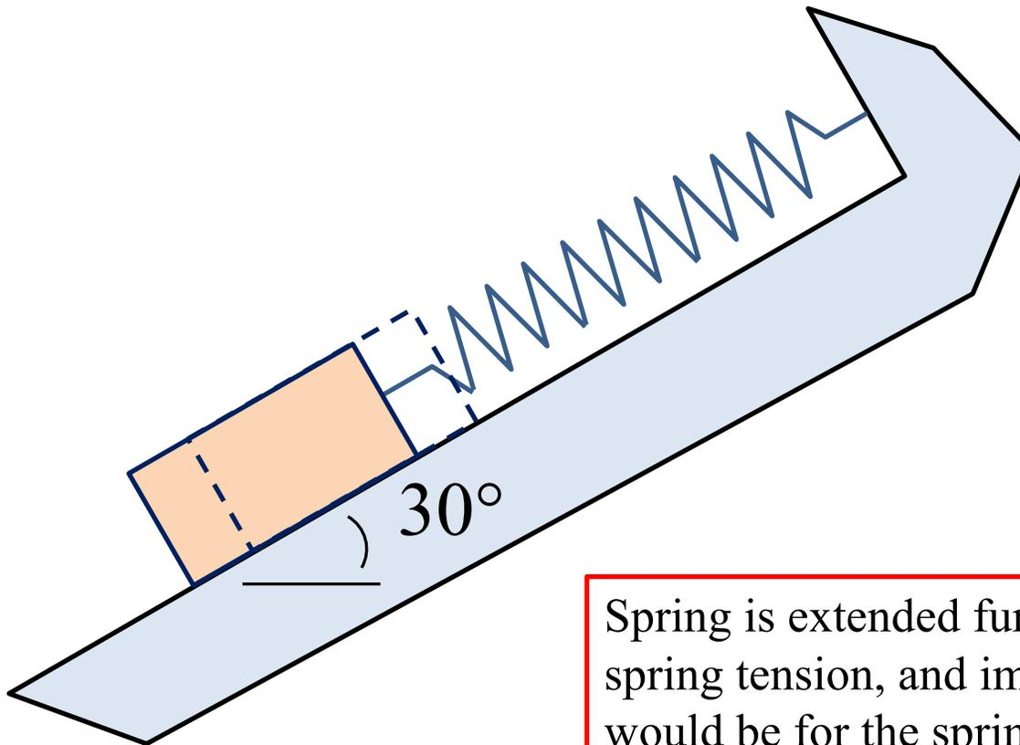
Spring is extended further, increasing spring tension, and impending motion would be for the spring to pull the crate up the incline.
