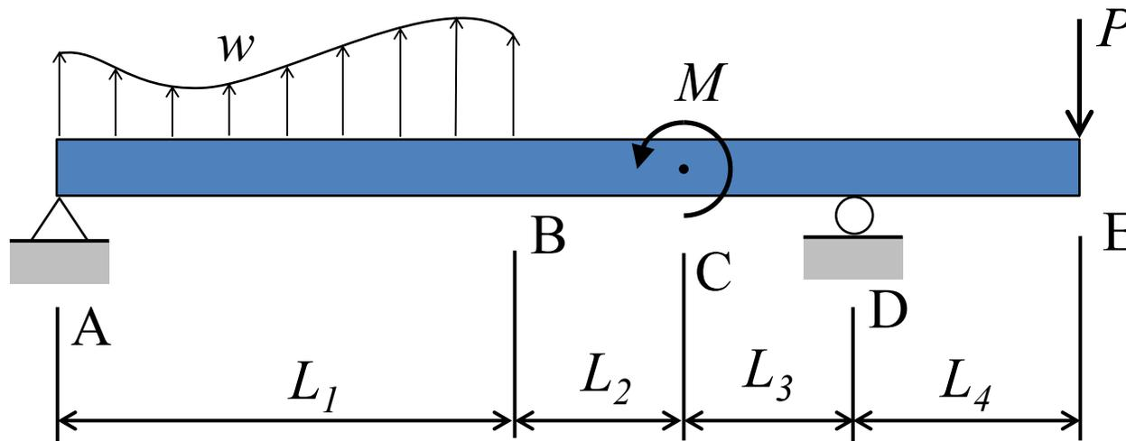
We would like to find the support reactions at the pin at A and roller at D
