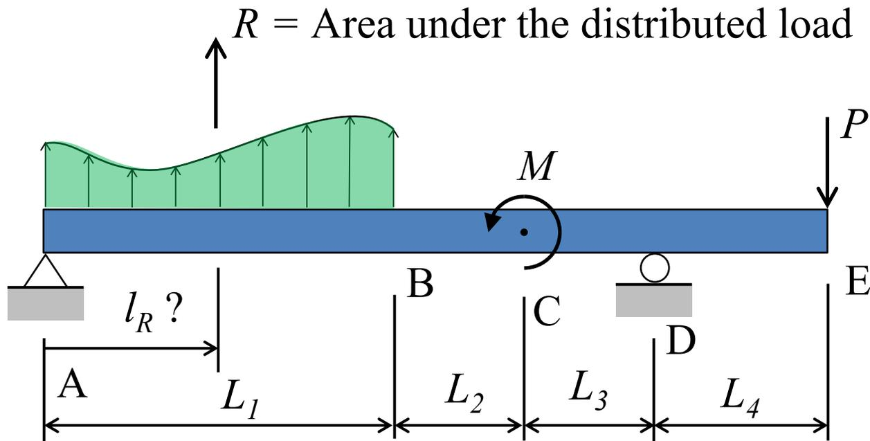
Where would we place the Equivalent point load to produce the same moment as the distributed load?
