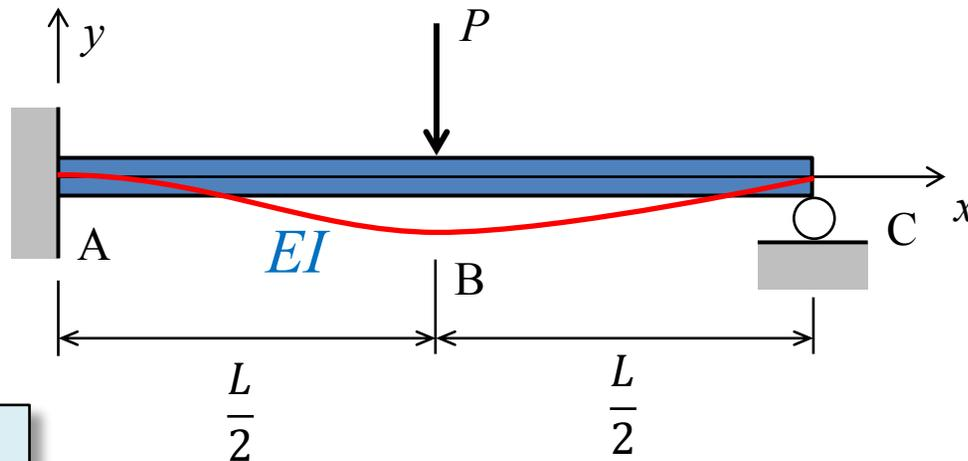
For the indeterminate beam subject to the point load,  $P$ , find the support reactions at A and C.  $EI$  is constant.
