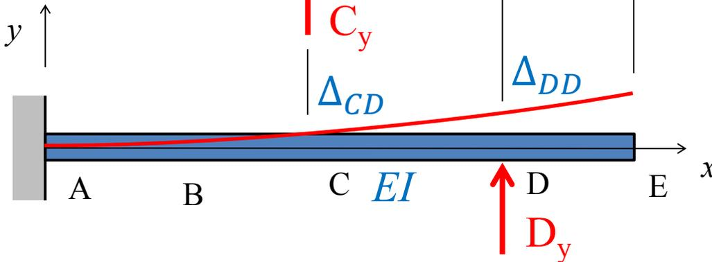
The Force Method is Based on the Principle of Superposition
