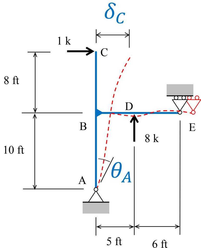
The statically determinate frame from our previous internal force diagram example is made up of columns that are W8x48 ( $I = 184 \text{ in}^4$ ) members and a beam that is a W10x22 ( $I = 118 \text{ in}^4$ ). The modulus of elasticity of structural steel is 29,000 ksi, which yields the following bending stiffnesses:
