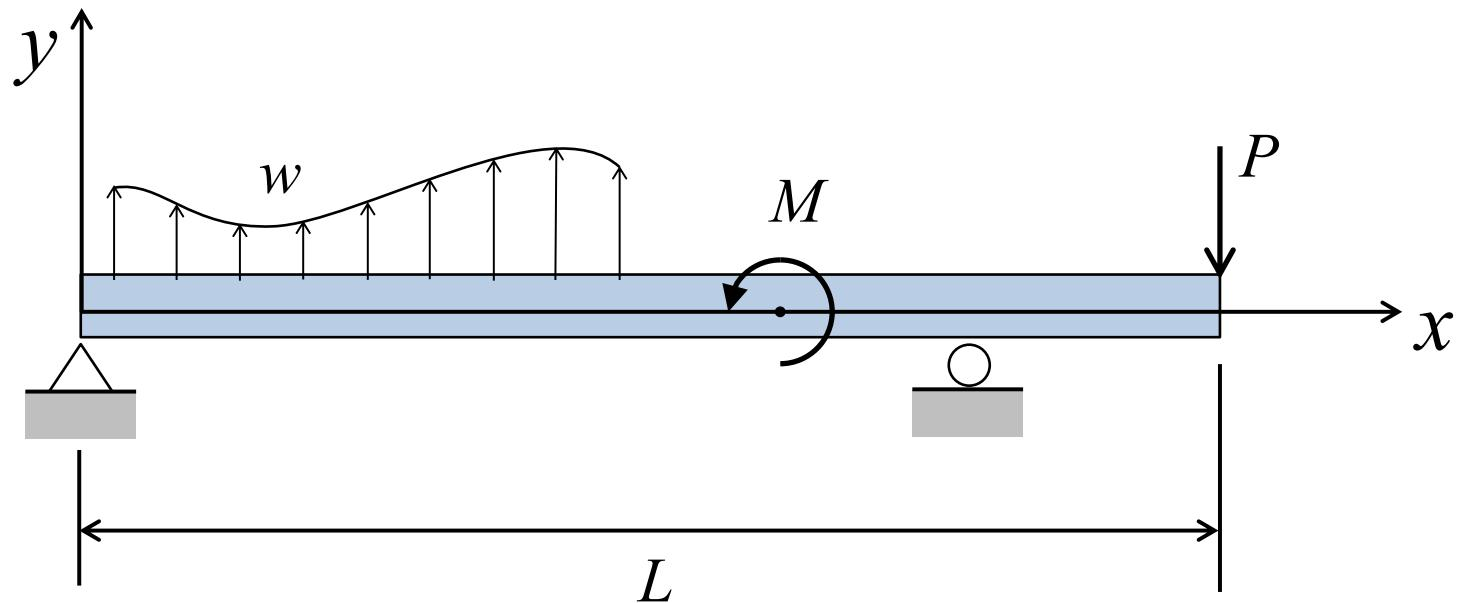
From an equilibrium analysis, find the internal bending moment function for the real system:
