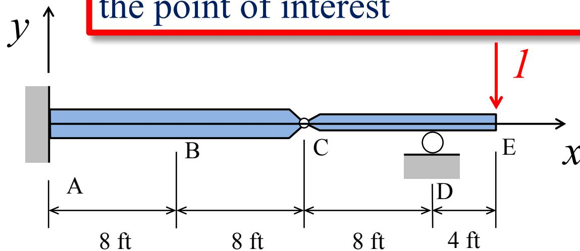
From an equilibrium analysis, find the internal bending moment function for the virtual system:
