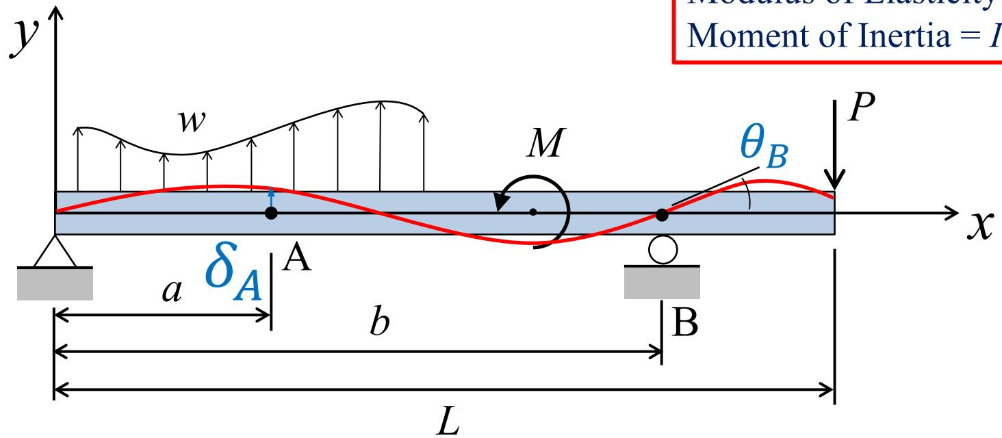
We want to find the deflection at point A and the slope at point B due to the applied loads
