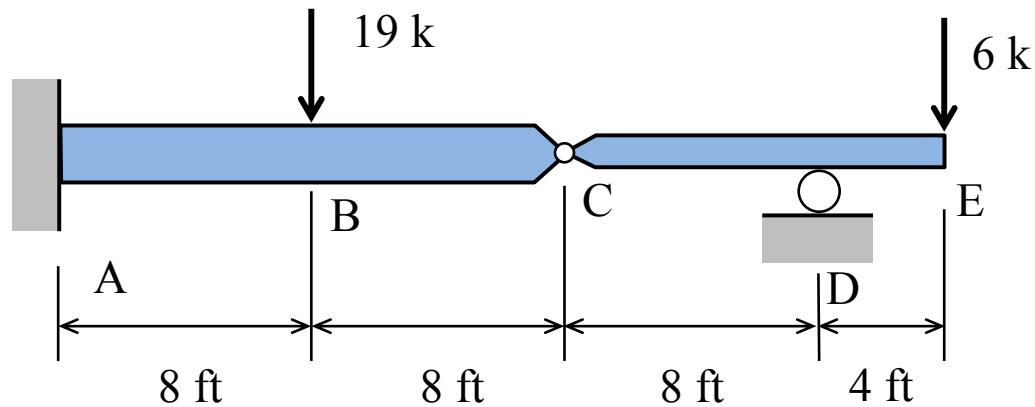
From an equilibrium analysis, find the internal bending moment function for the real system:
