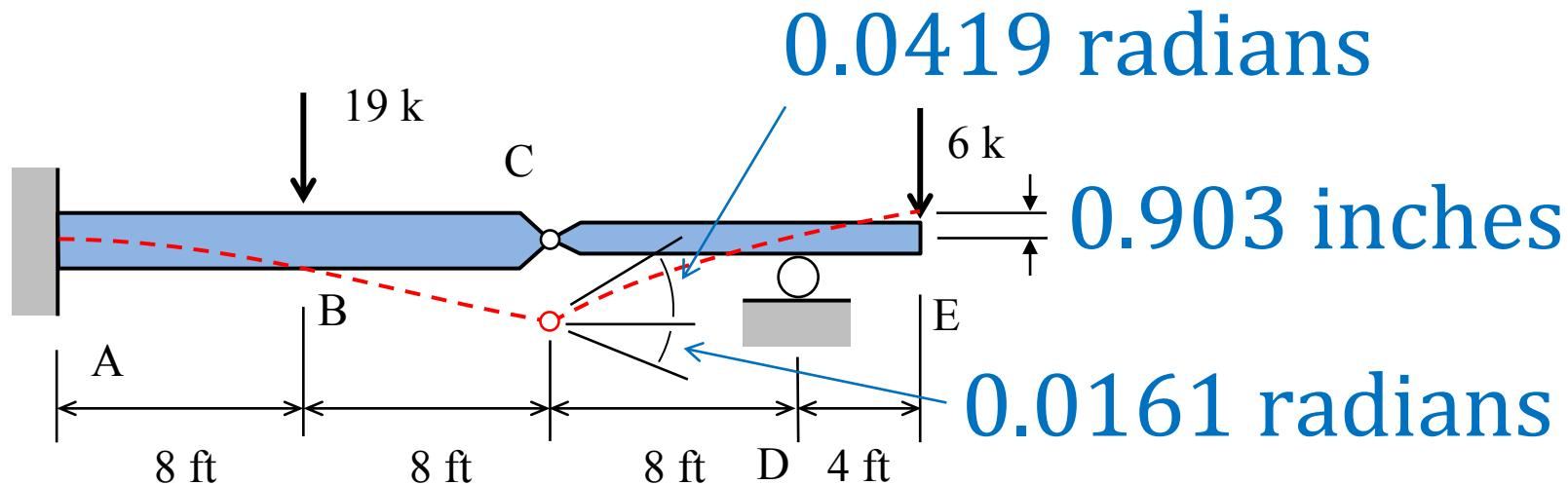
The overhanging beam shown has a fixed support at A, a roller support at C and an internal hinge at B.  $EI_{ABC} = 2,000,000 \text{ k-in}^2$  and  $EI_{CDE} = 800,000 \text{ k-in}^2$
