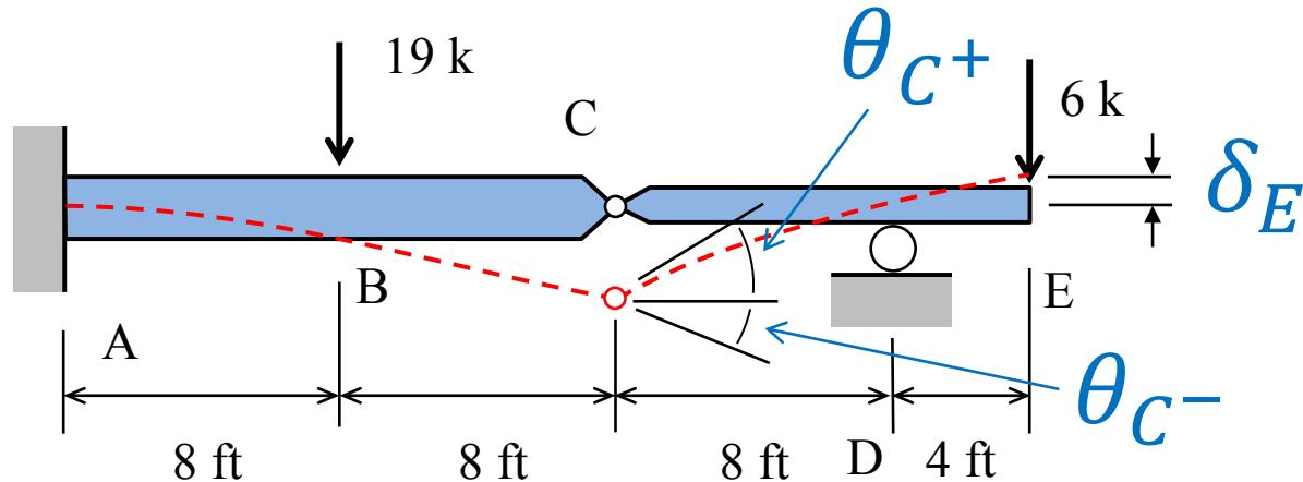
The overhanging beam shown has a fixed support at A, a roller support at C and an internal hinge at B.  $EI_{ABC} = 2,000,000 \text{ k-in}^2$  and  $EI_{CDE} = 800,000 \text{ k-in}^2$
