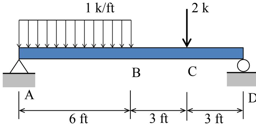
For the beam, which shear diagram is correct?
