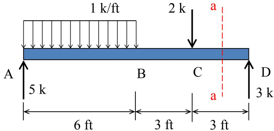
Consider the shear force at section a-a
