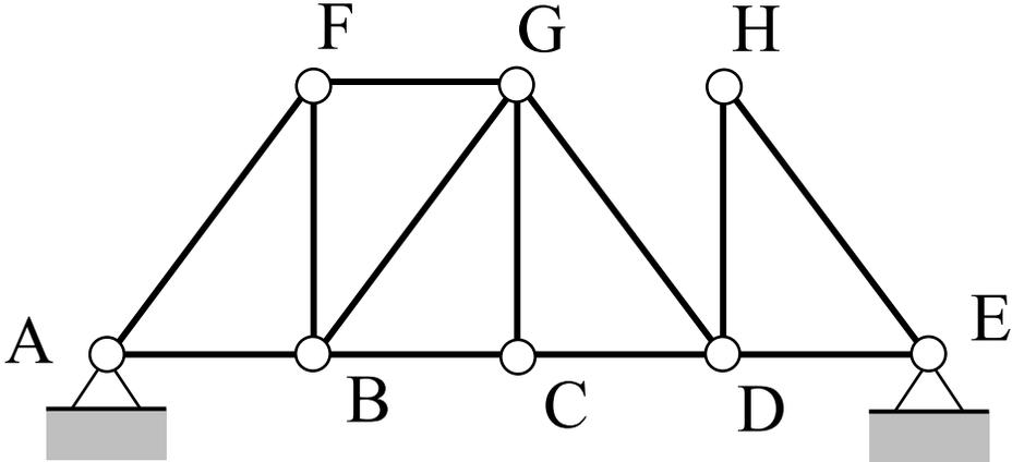
The truss shown has pin supports at A and E. Determine if the beam is stable under all possible loading conditions.
