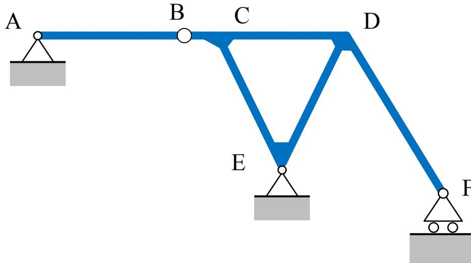
The stable frame shown has a roller support at F and pin supports at A and E. The frame members are rigidly connected at point C, D, and E and there is an internal hinge at B. If the frame is subjected to general loading, find the determinacy of the frame.
