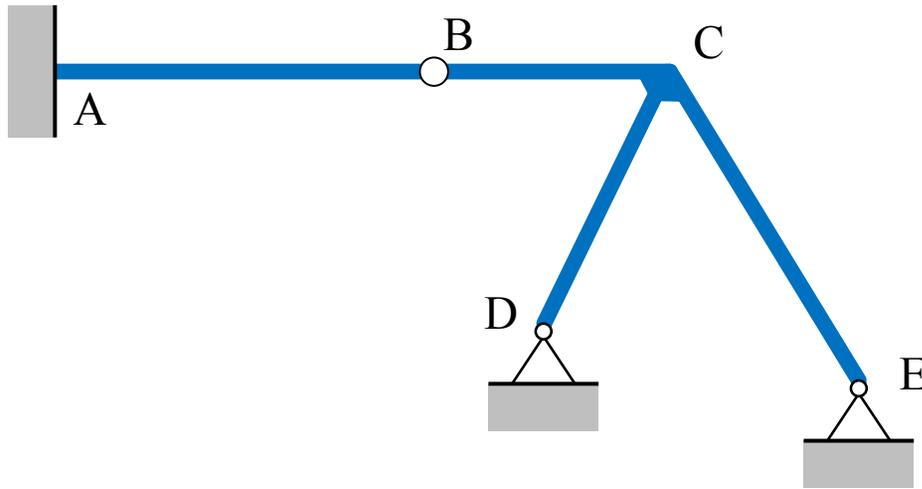
The stable frame shown has a fixed support at A and pin supports at D and E. The frame members are rigidly connected at point C and there is an internal hinge at B. If the frame is subjected to general loading, find the determinacy of the frame.
