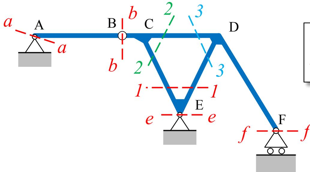
We must, at the minimum, cut the structure at the following locations and draw a FBD of each “piece” of the structure:
