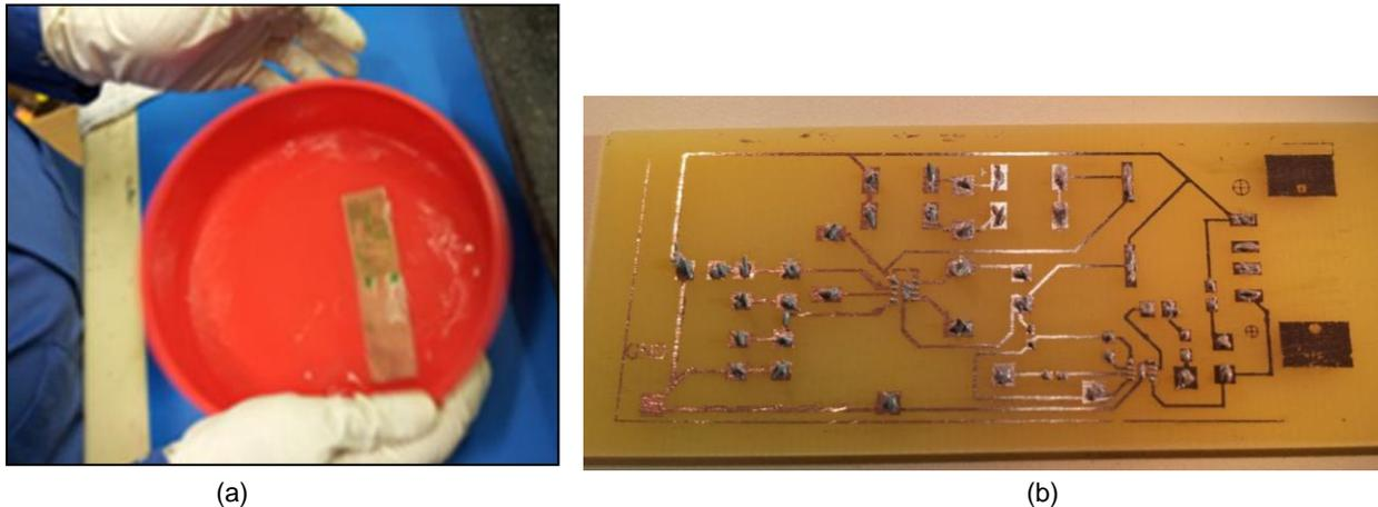
Figure 8: (a) Etching the board "at home". (b) Bare PCB with solder paste.
