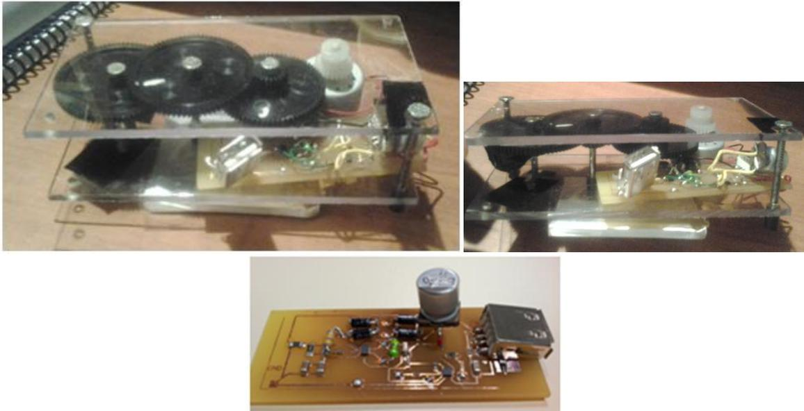
Figure 12: Final prototype of the DJYM. The case is taller than it should be due to the extra neck on the motor gear (can be seen in the one on the top right). The bottom is the final PCB with all components.
