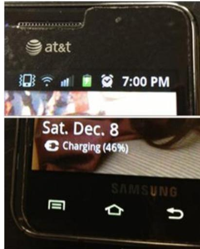
Figure 13: Using only the LTC3528 and manually spinning the gears, the phone can be charged. However, there is just enough power to slow down the depletion of the phone's battery power.
