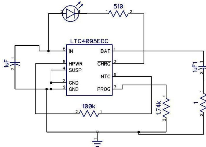
Figure 5: LTC4095 schematic
