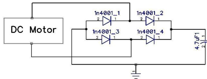
Figure 3: Schematic of a DC motor and full-wave rectifier circuit, with smoothing capacitor.
