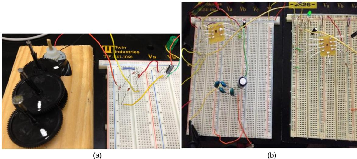
Figure 11: (a) First prototype of the gears was made on a wood block and outputs to the motor. (b) first prototype of the electrical components. The LTC3528, on the right outputs 5V. The LTC4095 is on the left.
