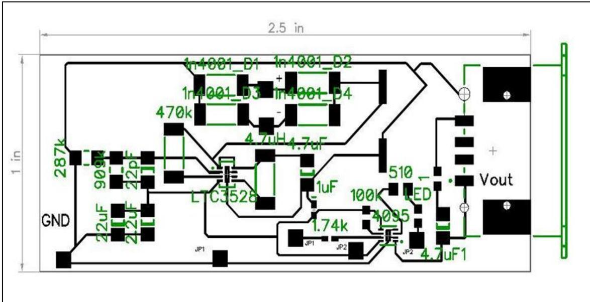
Figure 7: PCB layout
