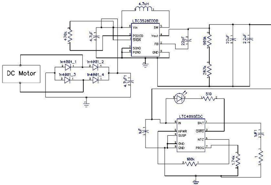
Figure 6: Full circuit diagram from gears to output.
