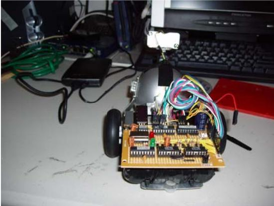
Fig 5: RoboVac's circuit picture
