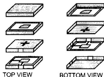
Fig. 1 – Physical layout of a 4-pole dual mode multilayer filter.
