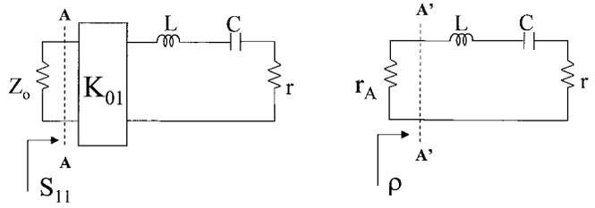
Fig. 1. Equivalent circuit of a series resonator.
