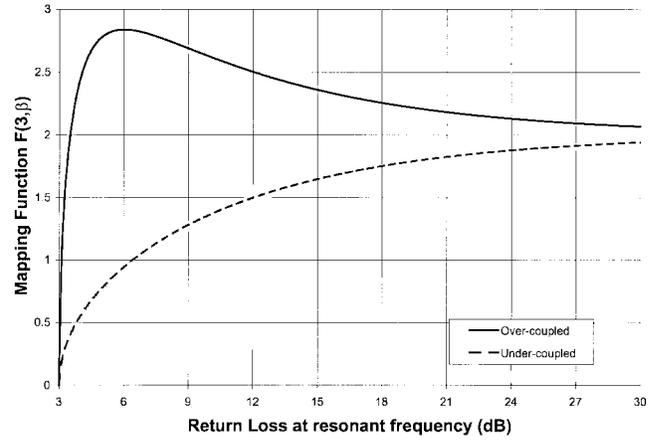
Fig. 3. Mapping function  $F(x, \beta)$  as a function of return loss at resonant frequency for  $x = 3$  dB.
