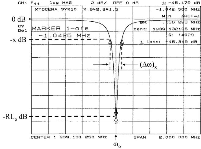
Fig. 2. A typical one-port  $|S_{11}|$  measurement of a microwave resonator. Shown here is the measured  $|S_{11}|$  for a dielectric resonator showing a  $Q_u$  of 32810.
