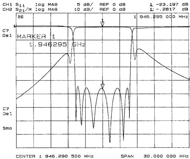
Fig. 5. Final performance of a 0.5% fractional bandwidth dielectric-resonator filter utilizing the described techniques. The realized unloaded  $Q$  of the filter is about 25000.
