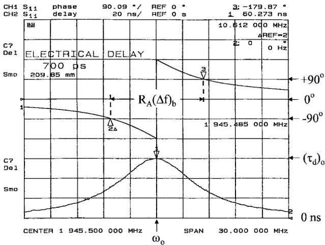
Fig. 4. Measured input coupling in terms of  $S_{11}$  phase and time delay for a 0.5% fractional bandwidth dielectrically loaded cavity filter. The electrical delay is adjusted so that (12) is valid.
