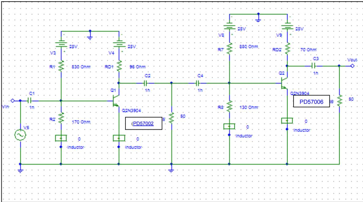
Figure 1: Schematic for Two Stage Amplifier Circuit for 30 dB Gain
