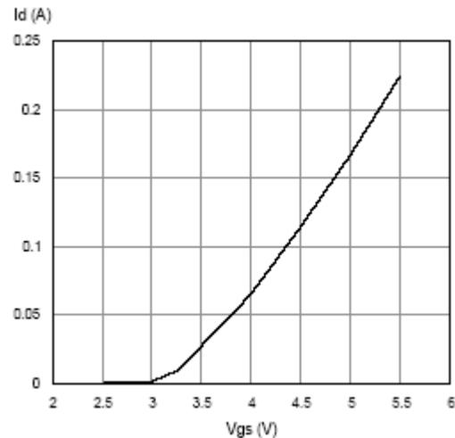
Figure 3:  $V_d$  Vs  $V_g$  curve for PD57002
