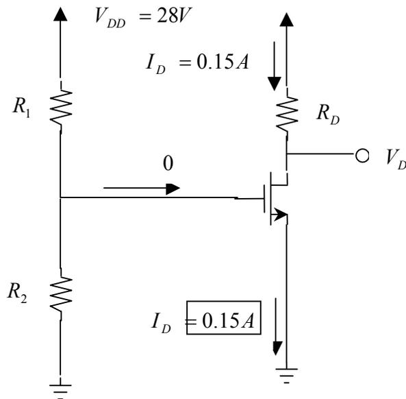
Figure 2: DC analysis circuit for [PD57002](#) and [PD57006](#)
