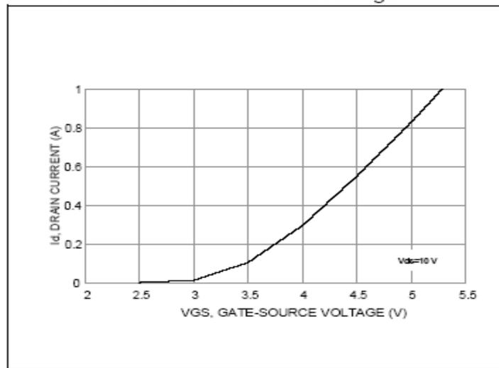
Figure 3:  $V_d$  Vs  $V_g$  curve for PD57006
