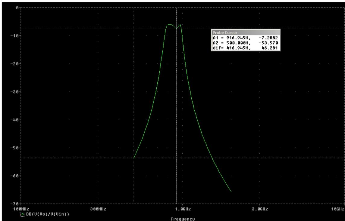
Fig. 3 The waveform of three order bandpass filter by real components
