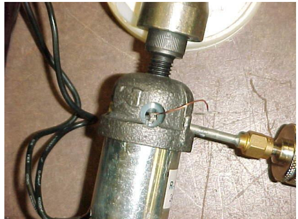
Fig II 12 : Electromagnet, ½” iron pipe and bolt pole piece, coax with ½ turn inductor at end, YIG sphere on rod (connected to wire for positioning) inserted in inductor
