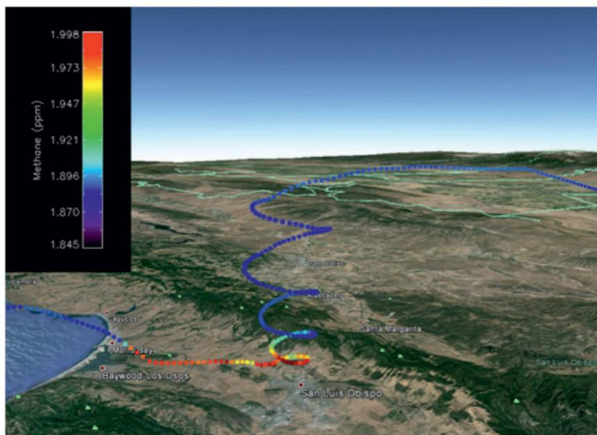
**FIG. 4. Methane mixing ratios measured on AJAX flight 116 (5 Mar 2014).**
