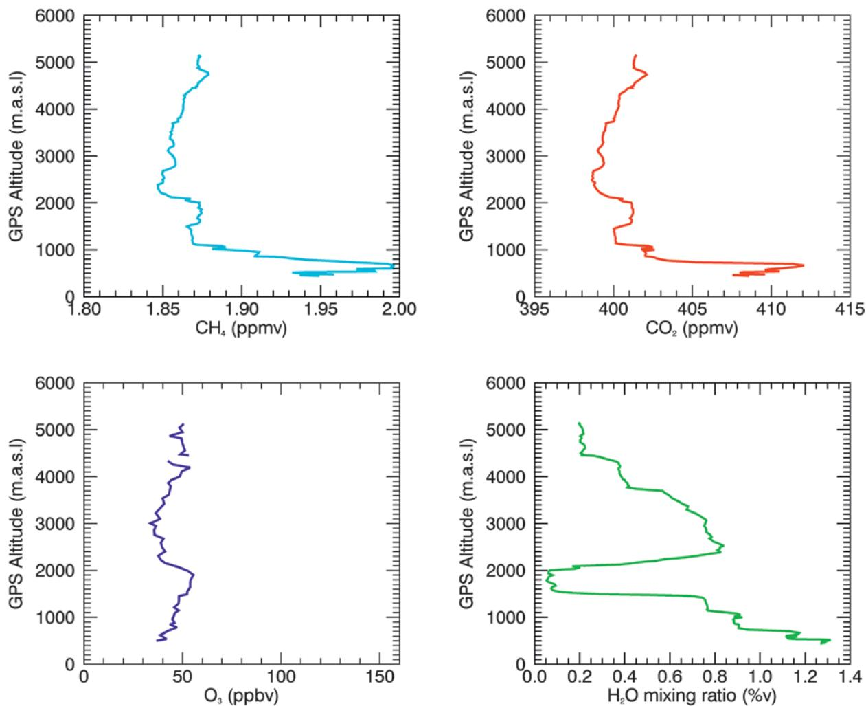
**FIG. 5. Profiles of methane, carbon dioxide, ozone, and water mixing ratio during the downward spiral over San Luis Obispo as obtained from Alpha Jet flight 116 (10-s averages for ozone; 3 s for methane, carbon dioxide, and water). Note the strong increases in methane and carbon dioxide at low altitudes.**
