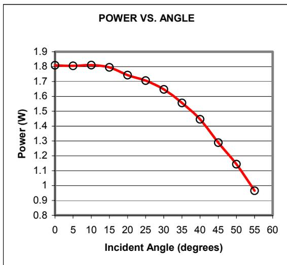
Figure 4. Power output vs. insolation angle for polycrystalline silicon solar panel [8].
