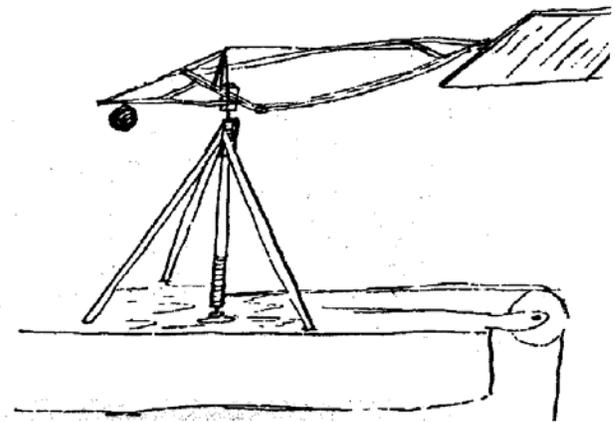
Figure 2. A whirling arm apparatus used by Sir George Cayley for measuring airfoil lift.
