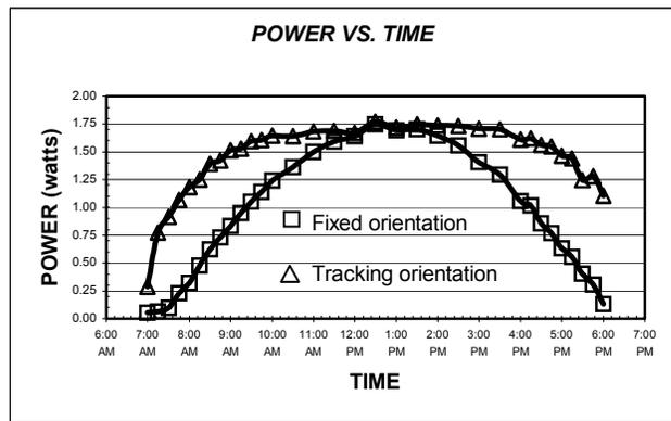
Figure 5. Power output for fixed orientation and tracking polycrystalline silicon solar panel [8].
