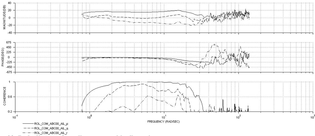
**Figure 22: Bode diagram for roll response with aileron input.**
