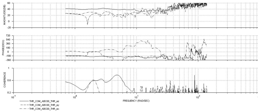
Figure 31: Throttle Bode/coherence plot
