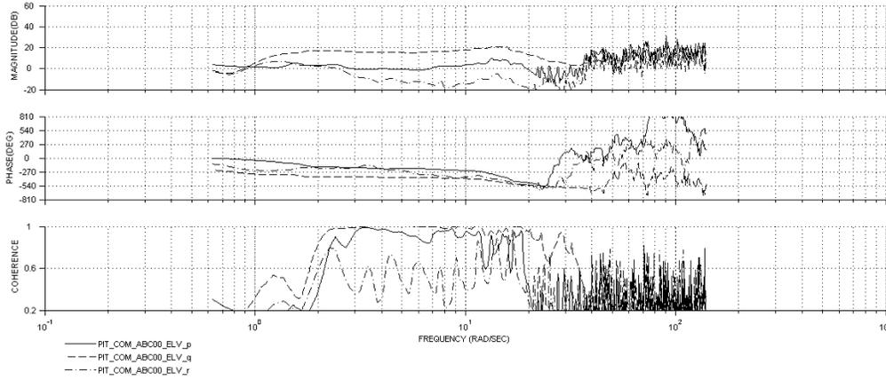
Figure 29: Pitch Bode/coherence plot
