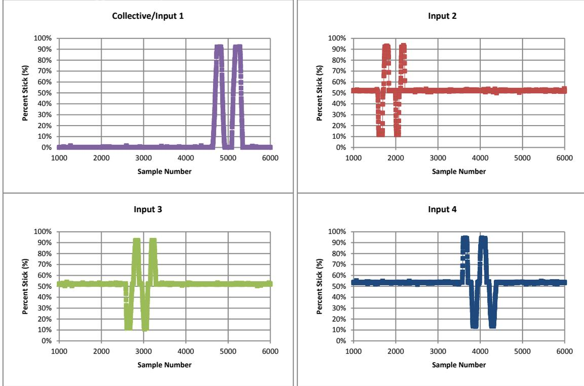
Figure 11: The controls check data is used to determine how the system identification unit records the input from the transmitter. In this case, the throttle, roll, pitch, and yaw commands correspond to inputs 1, 2, 3, and 4 respectively.
