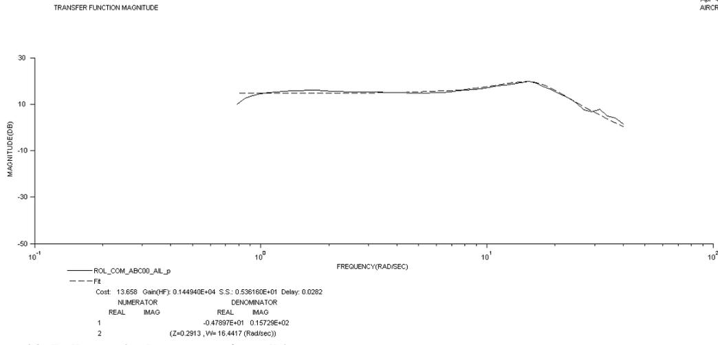
**Figure 23: Roll magnitude response for roll input.**
