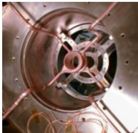
Figure 19 Actual ICRH antenna Source: Bering, 2006
