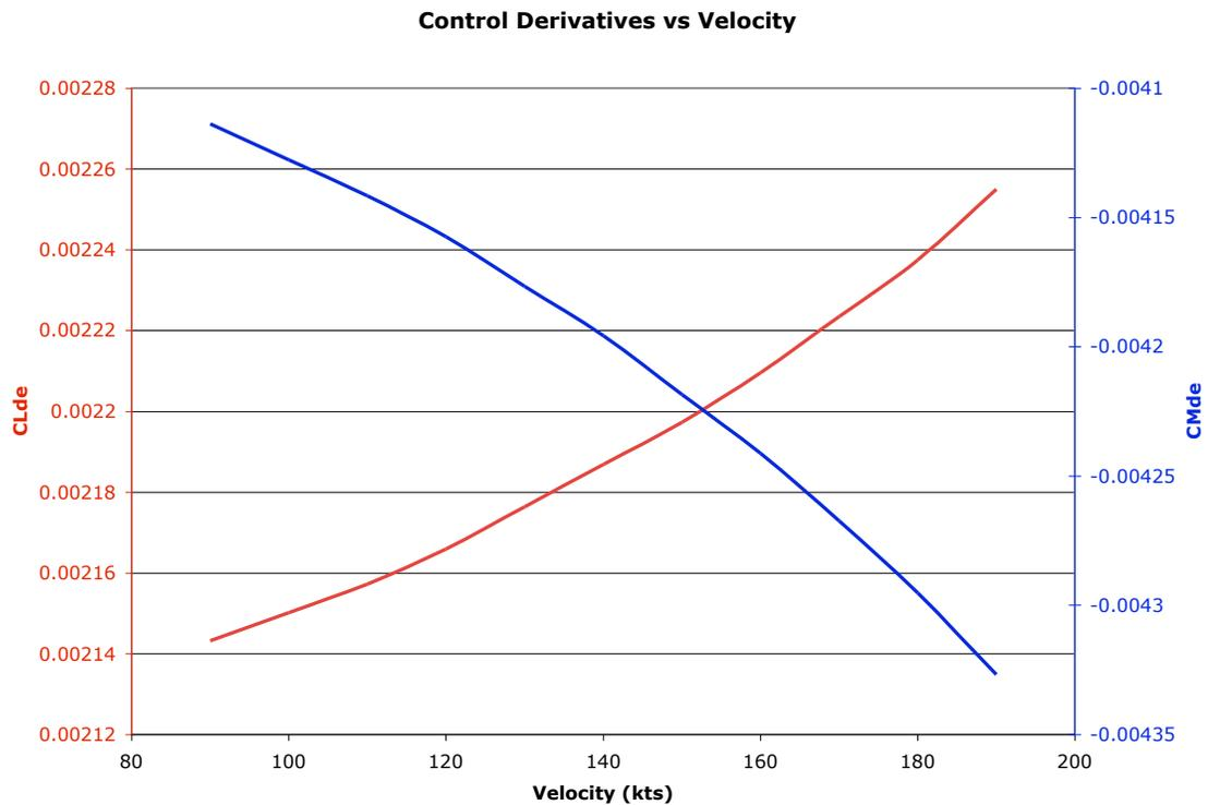
Figure 4.15. *Control Derivatives as a Function of Velocity*
