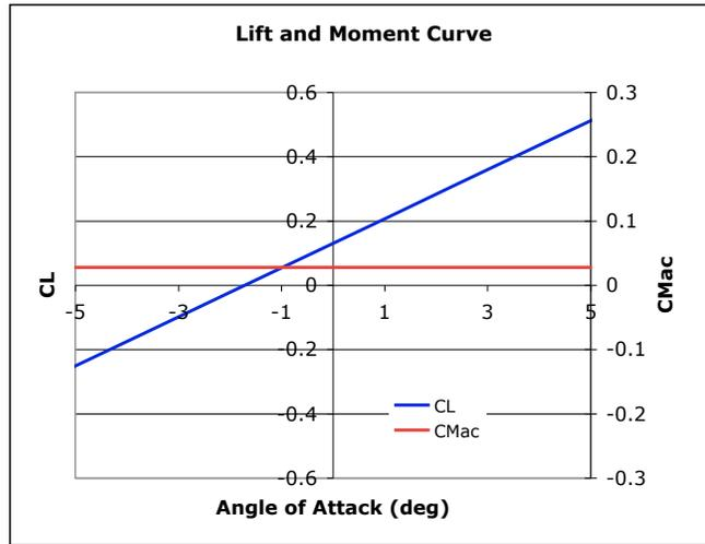
Figure 4.12. *Wing Lift and Moment Curve (Linear Range)*
