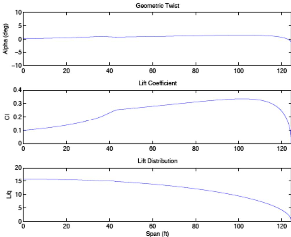
Figure 4.11. *Geometric Twist and Lift Distribution ( $\alpha = 0$ )*
