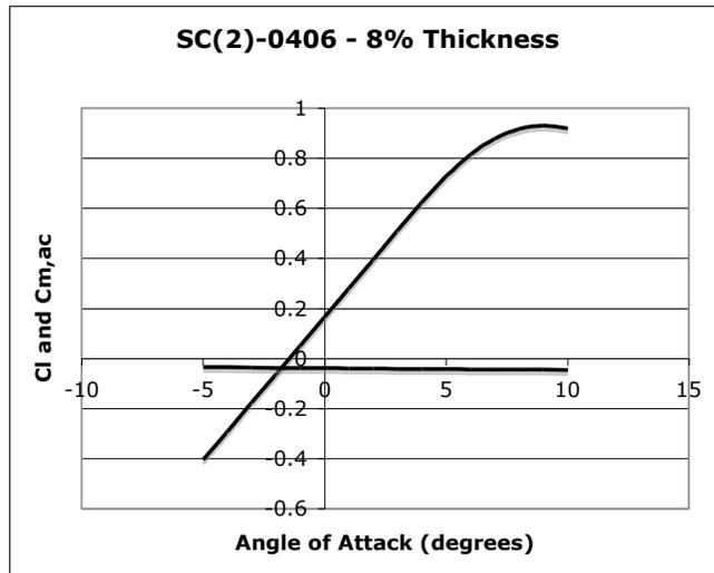
Figure 4.9. *SC(2)-0406 Lift and Moment Curve ( $Re=1 \times 10^8$ )*
