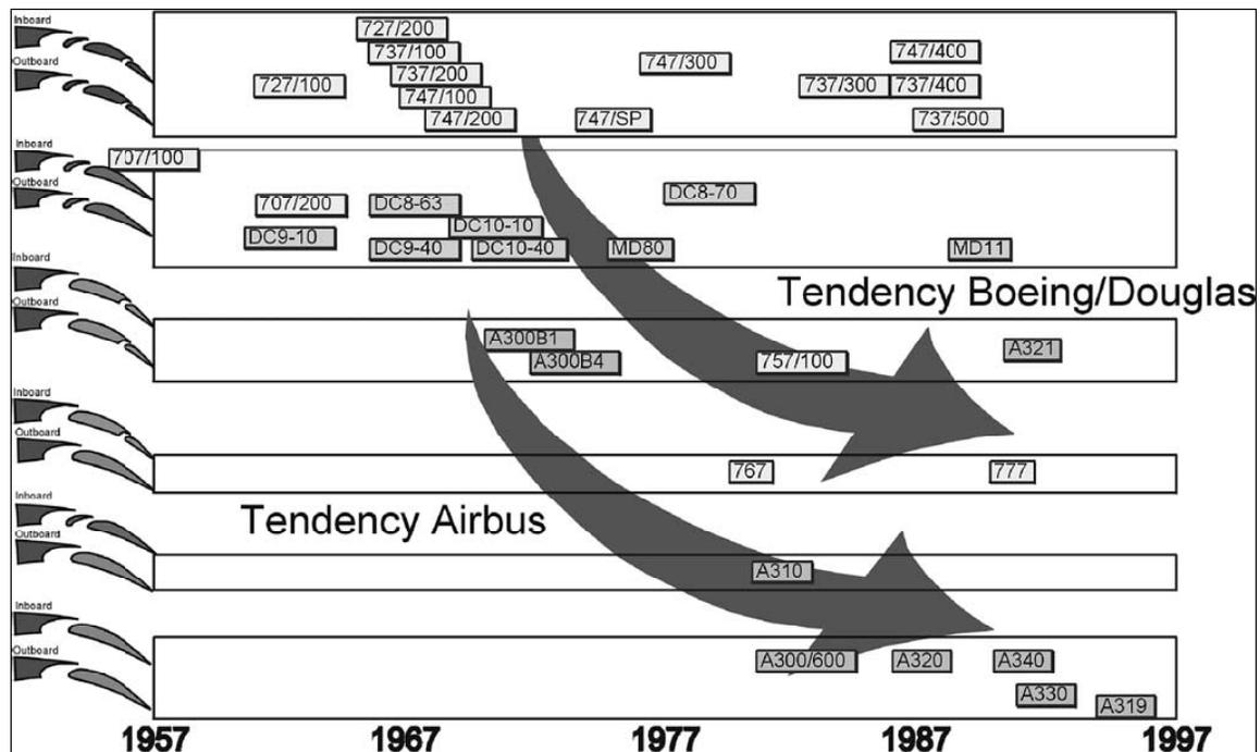
Figure 5.1. Design Evolution of Trailing Edge Devices [27]
