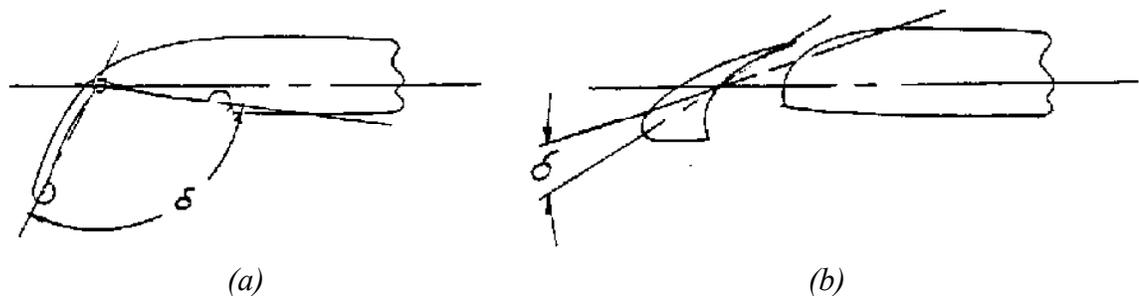
Figure 5.6. *Geometry of (a) Krueger Flap and (b) Slat [29]*
