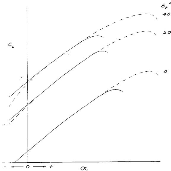
Figure 5.5. *Effect of Leading Edge Devices*
