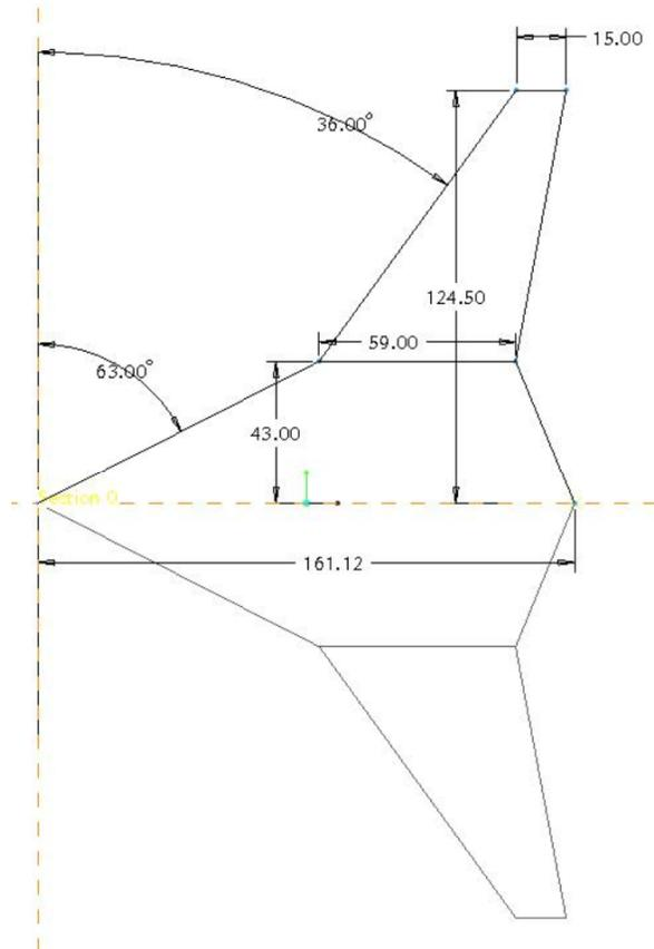
Figure 2.3. *Approximate Wing Geometry*
