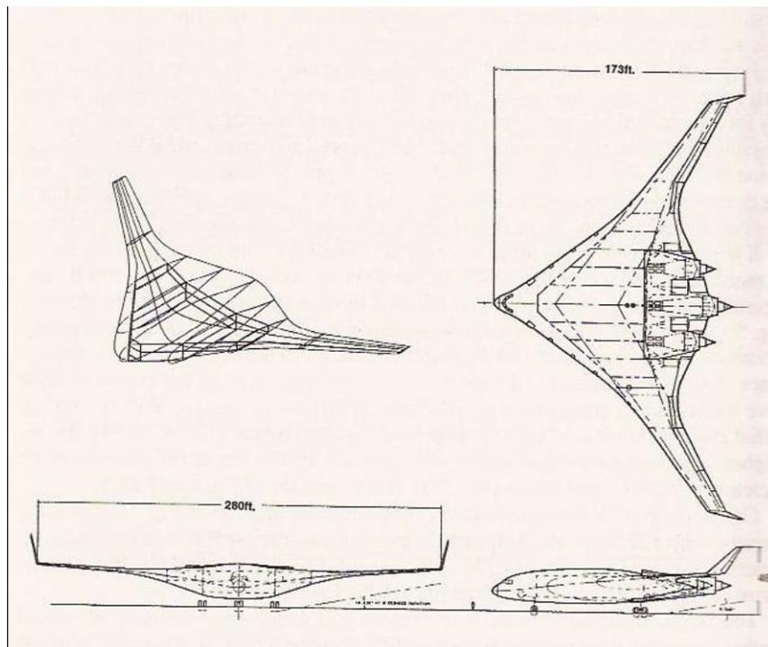
Figure 1.6. *Three View Drawing of 800 Passenger BWB Design [5]*
