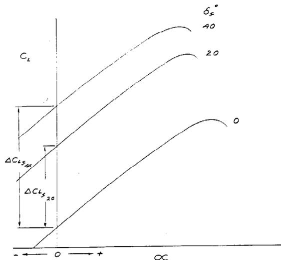
Figure 5.2. *General Effect of Trailing Edge Devices on Lift Curve Slope* [29]
