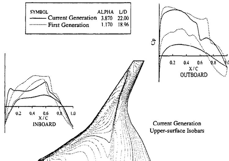
Figure 2.4. *Pressure Distributions For Inboard and Outboard Airfoils [2]*
