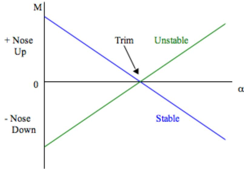
Figure 4.1. *Aircraft Pitching Moment vs Angle of Attack*
