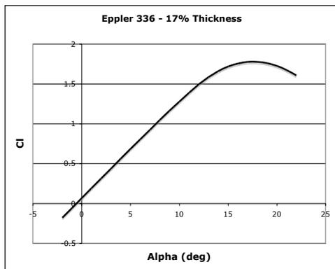
Figure 4.6. *Eppler 336 - Lift Curve ( $Re=1 \times 10^8$ )*
