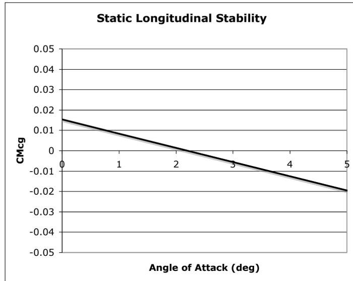
Figure 4.13. *Static Longitudinal Stability ( $C_{M,cg}$  vs.  $\alpha$ )*
