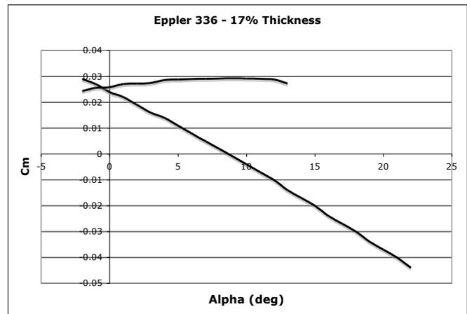
Figure 4.7. *Eppler 336 – Moment Curve ( $Re=1 \times 10^8$ )*
