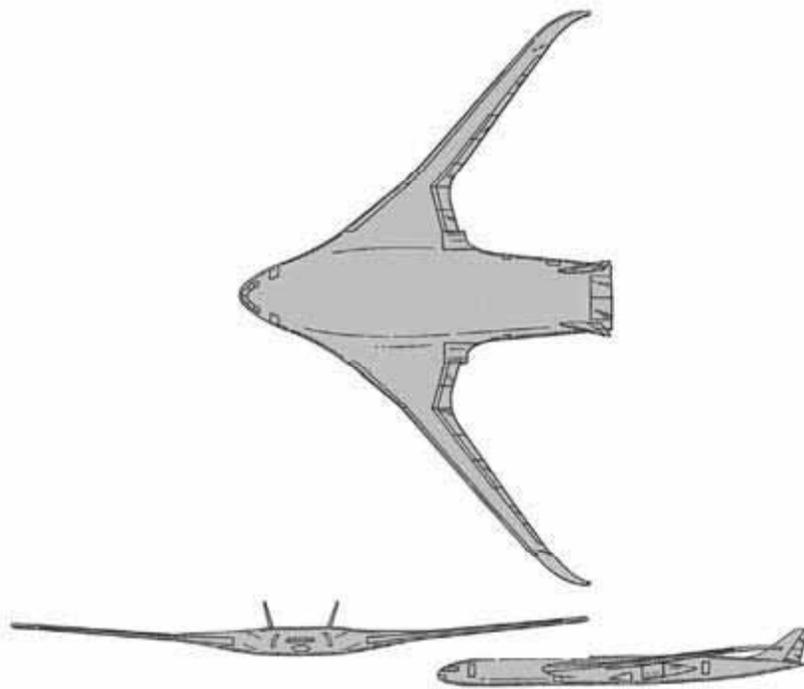
Figure 1.5. *First Generation Blended Wing Body* [4]
