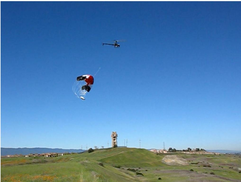
**Figure 38. Video capture of parafoil being lifted by the R/C helicopter for one of many drop tests.**
