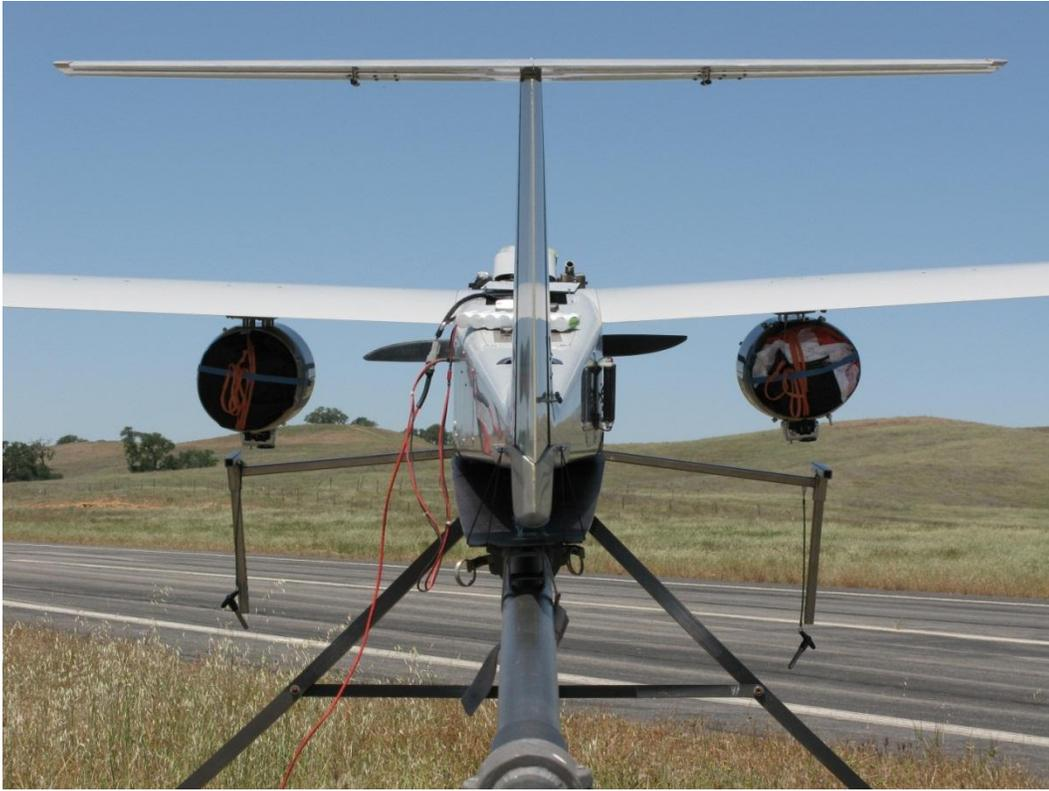
**Figure 41. System V.1 (left) and System V.2 (right) mounted to the wings of the UAV, ready for flight.**
