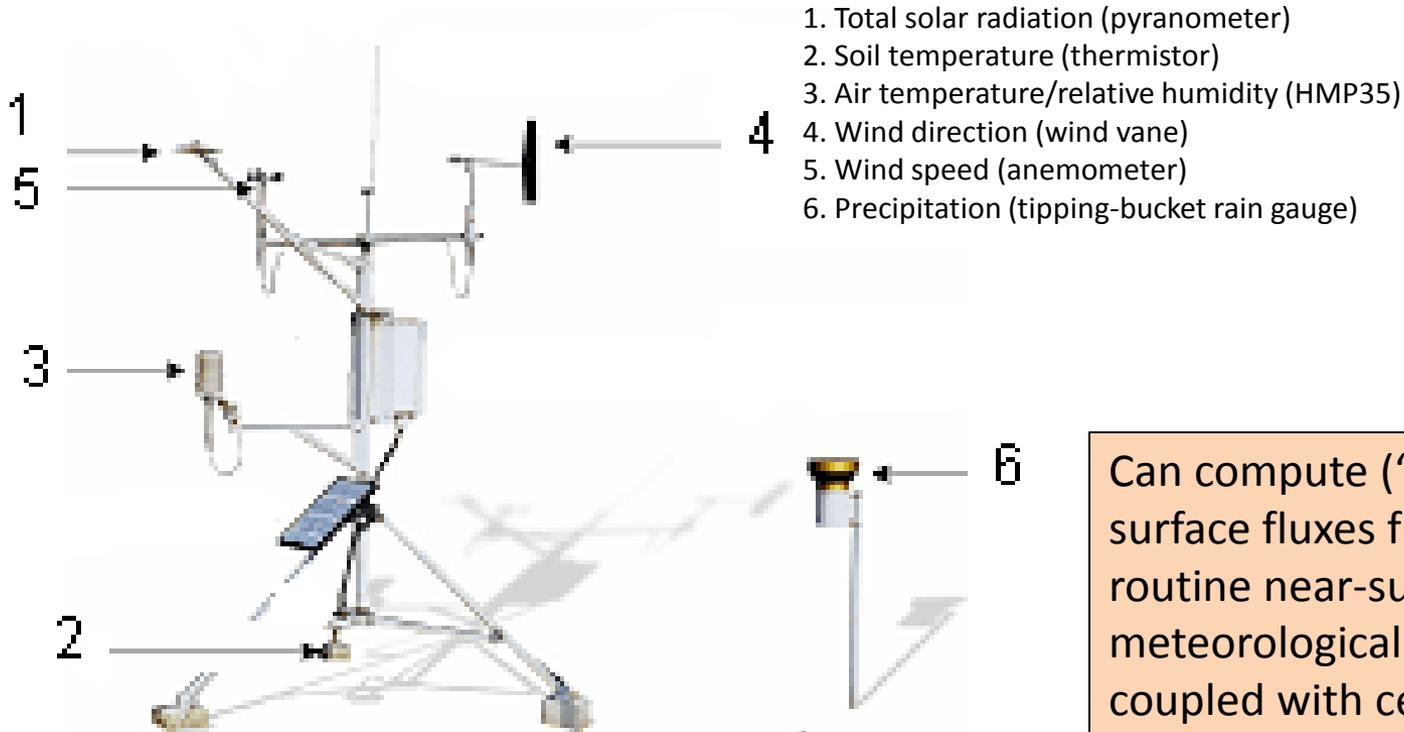
1. Total solar radiation (pyranometer)
