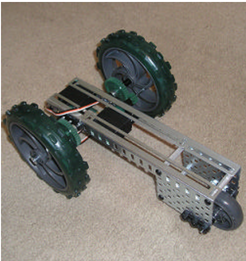
Drive wheels far from the center of gravity (CG), with significant drag from the castor.
